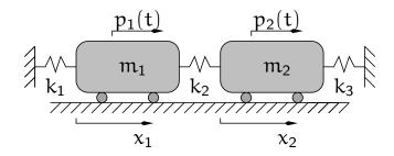
write the equation of equilibrium, using the D'Alembert principle, for each mass:
