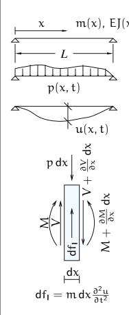
At the left, a straight beam with characteristic depending on position x: m = m(x) and EI = EI(x); with the signs conventions for displacements, accelerations, forces and bending moments reported left, the equation of vertical equilibrium for an infinitesimal slice of beam is
