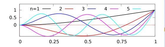
Above, in abscissas x/L and in ordinates  $\phi_n(x)$  for the first 5 modes of vibration of the cantilever beam.
