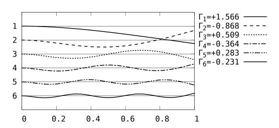
Above, the modal mass decomposition  $r_n = \Gamma_n m \phi_n$ , for the first six modes of a uniform cantilever, in abscissa  $\chi/L$ .
