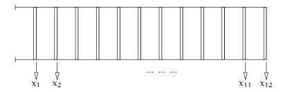
The structure above can be analyzed as a shear type building. The mass matrix is diagonal, with storey masses being all equal to m. The storey stiffnesses are linearly decreasing,  $k_1=23k,\ k_2=22k,\ ...,\ k_{11}=13k$  and  $k_{12}=12k$ . For example, the stifness matrix element  $k_{9,9}$  is given by  $k_{9,9}=k_9+k_{10}=29k$ .
