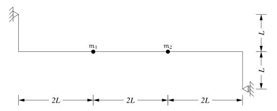
An uniform, simply supported beam substains two equal point masses, the beam mass being negligible with respect to the substained mass. Consider negligible also the axial and shear deformations of the beam.
