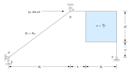
The articulated rigid system in figure is composed by two rigid bars,
