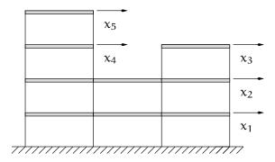
The structure depicted above can be analyzed as a shear type building. All columns are equal, each with a lateral stiffness indicated by k. One of the consequences of the previous statement is that the direct stiffness  $k_{11}$  is equal to 8k, because the number of column that must be deformed to have a unit displacement in  $x_1$  is 8.
