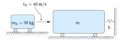
A body of mass  $m_b=30\,kg$  hits an undamped SDOF system, of unknown characteristics k and  $m_t$  with velocity  $\dot{x}_b=40\,m\,s^{-1}.$
