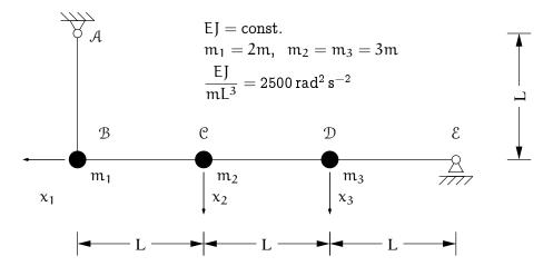
In the structure depicted above, the structural mass is negligible with respect to the masses of the three supported bodies, so it is correct to use the three DOF's in the figure as the dynamical degrees of freedom of the system.
