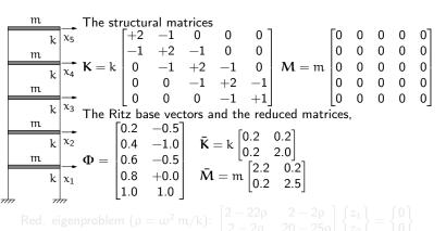
The roots are  $\rho_1=0.0824$ ,  $\rho_2=0.800$ , the frequencies are  $\omega_1=0.287\sqrt{k/m}~[=0.285]$ ,  $\omega_2=0.850\sqrt{k/m}~[=0.831]$ , exact solutions in [...].
