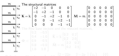
The roots are  $\rho_1=0.0824$ ,  $\rho_2=0.800$ , the frequencies are  $\omega_1=0.287\sqrt{k/m}~[=0.285],~\omega_2=0.850\sqrt{k/m}~[=0.831],$  exact solutions in  $[\ldots]$ .
