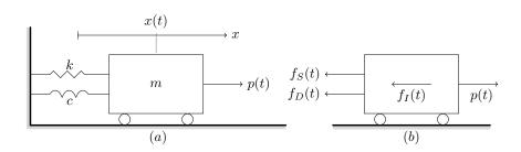
The equation of motion can be written using the D'Alembert Principle, expressing the equilibrium of all the forces acting on the mass including the inertial force.
