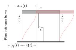
Displacements, deformations and stresses in a structure are induced also by a motion of its support.
