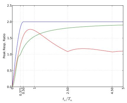
rectangular triangular half sine SDOF linear oscillator
