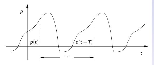
Periodic loadings can be expressed as an infinite series of harmonic functions using Fourier theorem, e.g., an antisymmetric loading is
