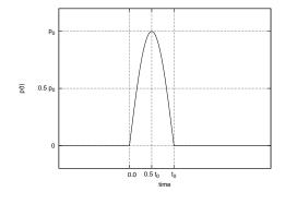
where  $\omega=\frac{2\pi}{2t_0}$  is the frequency associated with the load. Note that  $\omega$   $t_0=\pi$ .
