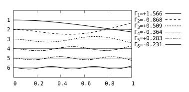
Above, the modal mass decomposition  $r_n = \Gamma_n m \phi_n$ , for the first six modes of a uniform cantilever, in abscissa  $\chi/L$ .
