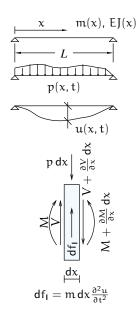
At the left, a straight beam with characteristic depending on position x: m = m(x) and EJ = EJ(x); with the signs conventions for displacements, accelerations, forces and bending moments reported left, the equation of vertical equilibrium for an infinitesimal slice of beam is
