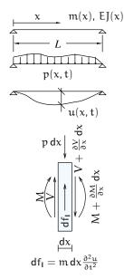
At the left, a straight beam with characteristic depending on position x: m = m(x) and EJ = EJ(x); with the signs conventions for displacements, accelerations, forces and bending moments reported left, the equation of vertical equilibrium for an infinitesimal slice of beam is
