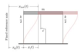
Considering a support motion  $x_g(t)$ , defined with respect to a inertial frame of reference, the total displacement is
