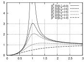
It is possible to measure the support displacement measuring the deflection of the oscillator, within an almost constant scale factor, for excitation frequencies larger than  $\omega_n$ .
