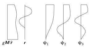
For EQ loading,  $\Gamma_1$  is relatively large for the first mode, as loading components and displacements have the same sign, with respect to other  $\Gamma_i$ 's, where the oscillating nature of the higher eigenvectors will lead to increasing cancellation. On the other hand, consider the external loading, whose peculiar shape is similar to the 3rd mode.  $\Gamma_3$  will be more relevant than  $\Gamma_i$ 's for lower or higher modes.
