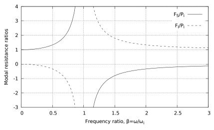
For a fixed excitation frequency and high modal frequencies the frequency ratio  $\beta \to 0$ .
