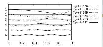
Above, the modal mass decomposition  $r_n = \Gamma_n m \varphi_n$  ,for the first six modes of a uniform cantilever, in abscissa x/L.
