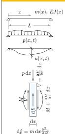
At the left, a straight beam with characteristic depending on position x: m = m(x) and EJ = EJ(x); with the signs conventions for displacements, accelerations, forces and bending moments reported left, the equation of vertical equilibrium for an infinitesimal slice of
