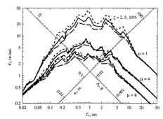
El Centro 1940 NS, elastic response spectra and inelastic spectra for  $\mu=4$  and  $\mu=8,$  for different values of  $\zeta$  (2%, 5% and 10%). Effects of damping are relatively important and only in the velocity controlled area of the spectra, while effects of ductility are always important except in the high frequency range.
