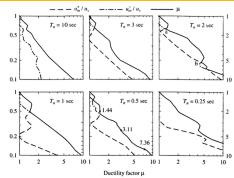
On the left, for different  $T_n$ 's and  $\mu = 5\%$ . the indipendent variable is in the ordinates, either  $\bar{f}_y$  (left) or  $R_y$  (rigth) the strength reduction factor. Dash-dash lines is  $u_m^+/u_y$ , dash-dot is  $u_m^-/u_y$ .
