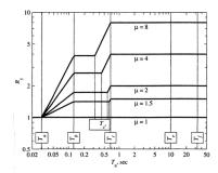
Based on observations and energetic considerations, the plots of  $R_y$  vs  $T_n$  for different  $\mu$  values can be approximated with straight lines in a log-log diagram, where the constant pieces are defined in terms of the key periods in D-V-A graphs.
