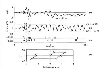
The various response graphs above were computed for  $\bar{f}_y = 0.125$ (i.e.,  $R_y=8$  and  $f_y=\frac{1.37}{8}$ w=0.171w) and  $\zeta=0$ ,  $T_n=0.5$ s.
