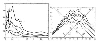
On the left, a lin-lin plot of the pseudo-acceleration normalized (and adimensionalised) with respect to g, the acceleration of gravity.
