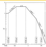
One storey frame, weight w, period is  $T_n = 0.25 \,\mathrm{s}$ , damping ratio is  $\zeta=5\%$ , peak ground acceleration is  $\ddot{x}_{g0} = 0.5\,\mathrm{g}$ . Find design forces for 1) system remains elastic, 2)  $\mu = 4$  and 3)  $\mu = 8$ . In the figure, a reference elastic spectrum for  $\ddot{x}_{g0}=1\,\mathrm{g}$ ,  $A_y(0.25) = 2.71\,\mathrm{g}; \ \mathrm{for}$  $\ddot{x}_{g0}=0.5\,\mathrm{g} \ \mathrm{it} \ \mathrm{is} \ f_0=1.355w.$
