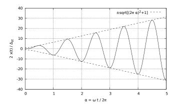
$$\frac{2}{\Delta_{\rm st}}x(t) = \sin \omega t - \omega t \cos \omega t = \sin 2\pi \alpha - 2\pi \alpha \cos 2\pi \alpha.$$
