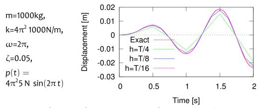
It is apparent that you have a very good approximation when the linearised loading is a very good approximation of the input function, let's say  $h \le T/10$ .
