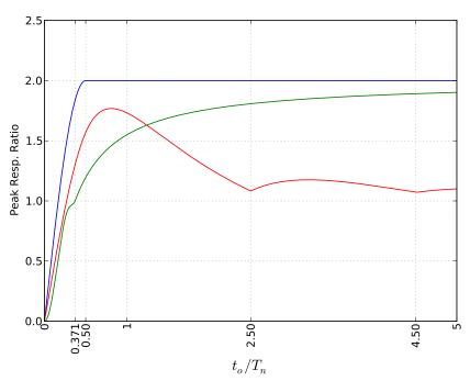
rectangular triangular half sine SDOF linear oscillator
