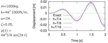
It is apparent that you have a very good approximation when the linearised loading is a very good approximation of the input function, let's say  $h \le T/10$ .
