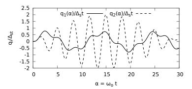
In the graph above, the responses are plotted against an adimensional time coordinate  $\alpha$  with  $\alpha=\omega_0 t$ , while the ordinates are adimensionalised with respect to  $\Delta_{\rm st}=\frac{p_0}{l}$
