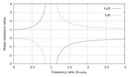
For a fixed excitation frequency and high modal frequencies the frequency ratio  $\beta \rightarrow 0$ .
