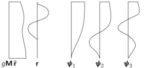
For EQ loading,  $\Gamma_1$  is relatively large for the first mode, as loading components and displacements have the same sign, with respect to other  $\Gamma_i$ 's, where the oscillating nature of the higher eigenvectors will lead to increasing cancellation. On the other hand, consider the external loading, whose peculiar shape is similar to the 3rd mode.  $\Gamma_3$  will be more relevant than  $\Gamma_i$ 's for lower or higher modes. Truncation Errors, Correction Procedures
