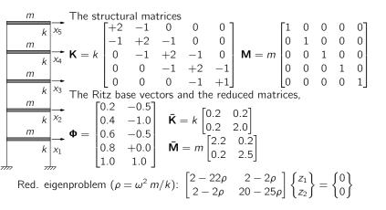
The structural matrices  $\pi\pi$ Red. eigenproblem  $(\rho = \omega^2 m/k)$ :  $\begin{bmatrix} 2 - 22\rho & 2 - 2\rho \\ 2 - 2\rho & 20 - 25\rho \end{bmatrix} \begin{cases} z_1 \\ z_2 \end{cases} = \begin{cases} 0 \\ 0 \end{cases}$ The roots are  $\rho_1 = 0.0824$ ,  $\rho_2 = 0.800$ , the frequencies are  $\omega_1 = 0.287 \sqrt{k/m}$  [ = 0.285],  $\omega_2 = 0.850 \sqrt{k/m}$  [ = 0.831], while the
