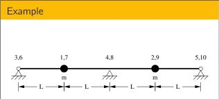
The dynamic *DOF* are  $x_1$  and  $x_2$ , vertical displacements of the two equal masses,  $x_3$ ,  $x_4$ ,  $x_5$  are the imposed vertical displacements of the supports,  $x_6, \ldots, x_{10}$  are the rotational degrees of freedom (removed by static condensation).
