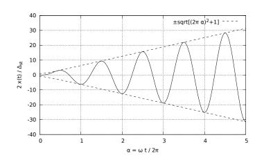
$$\frac{2}{\Delta}x(t) = \sin \omega t - \omega t \cos \omega t = \sin 2\pi \alpha - 2\pi \alpha \cos 2\pi \alpha.$$
