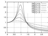
1. For  $\beta<\sqrt{2}$ , TR is always greater than 1: the transmitted force is amplified. 2. For  $\beta>\sqrt{2}$ , TR is always smaller than 1 and for the same  $\beta$  TR decreases with  $\zeta$ .
