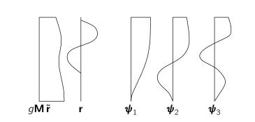
For EQ loading,  $\Gamma_1$  is relatively large for the first mode, as loading components and displacements have the same sign, with respect to other  $\Gamma_i$ 's, where the oscillating nature of the higher eigenvectors will lead to increasing cancellation. On the other hand, consider the external loading, whose peculiar shape is similar to the 3rd mode.  $\Gamma_3$  will be more relevant than  $\Gamma_i$ 's for lower or higher modes.
