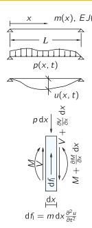
m(x), EJ(x) At the left, a straight beam with characteristic depending on position x: m=m(x) and EJ=EJ(x); with the signs conventions for displacements, accelerations, forces and bending moments reported left, the equation of vertical equilibrium for an infinitesimal slice of beam is
