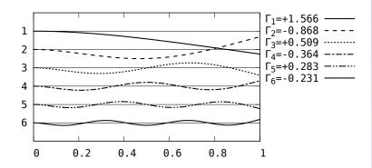
Above, the modal mass decomposition  $r_n = \Gamma_n m \phi_n$ , for the first six modes of a uniform cantilever, in abscissa x/L.
