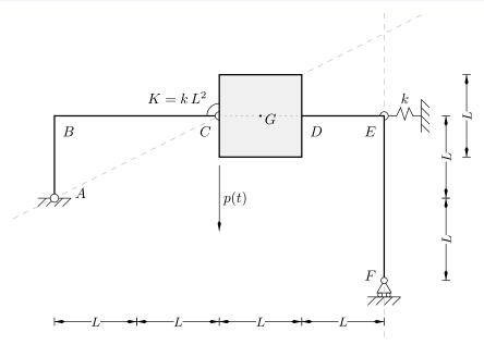
The left body being 1 and the right one being 2, the Centres of Instantaneous Rotations  $\Omega_1$  and  $\Omega_2$  are the hinge in A and the intersection of the dotted lines.
