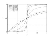
$\theta(\beta,\zeta)$  has a sharper variation around  $\beta=1$  for decreasing values of  $\zeta$ , but it is apparent that, in the case of slightly damped structures, the response is approximately in phase for low frequencies of excitation, and in opposition for high frequencies. It is worth mentioning that for  $\beta=1$  we have that the response is in perfect quadrature with the load: this is very important to detect resonant response in dynamic tests of structures.
