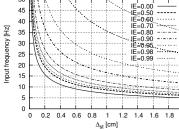
Knowing the frequency of excitation and the required level of vibration isolation efficiency (IE), one can determine the minimum static deflection (proportional to the spring flexibility) required to achieve the required IE. It is apparent that any isolation system must be very flexible to be effective.
