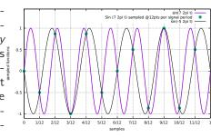
See the plot above: the contributions from the high frequency sines, when sampled, are indistinguishable from the contributions from lower frequency components, i.e., are *aliased* to lower frequencies!
