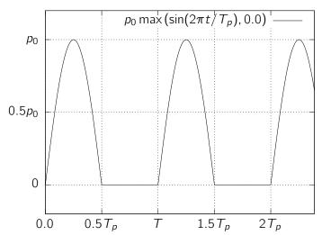
As an example, consider the loading  $p(t) = \max\{p_0 \sin \frac{2\pi t}{T_0}, 0\}$
