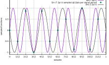
See the plot above: the contributions from the high frequency sines, when sampled, are indistinguishable from the contributions from lower frequency components, i.e., are aliased to lower frequencies!
