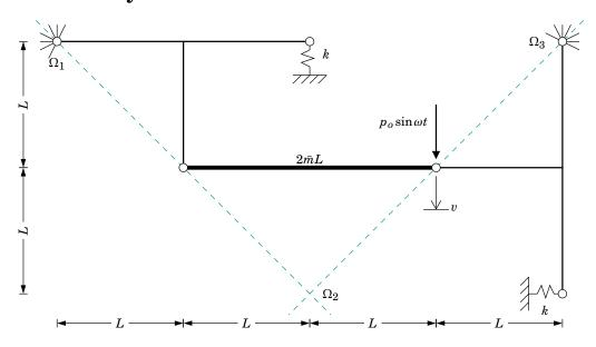
The SDOF system in figure is composed of 3 rigid bodies and 2 elastic springs of equal stiffness k and it is excited by a vertical force,  $p(t) = p_o \sin \omega t$ , applied to the right internal hinge. Only the central body has a significant mass.
