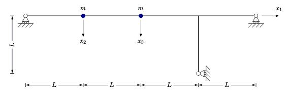
The system in figure is composed of a single uniform beam, supporting two equal lumped masses and you can assume that
