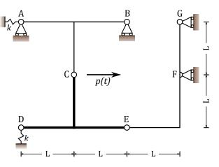
The system in figure is composed of three rigid bars, two elastic springs and four rollers and it is loaded by a time varying force p(t),
