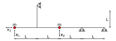
Considering that the mass of the beam is negligible with respect to the lumped masses and that the axial and shear deformations are negligible with respect to the flexural ones, you can use a 3 DOF system to investigate the dynamic behaviour of the system.
