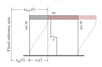
Considering a support motion  $x_{\rm g}(t)$ , defined with respect to a inertial frame of reference, the total displacement is
