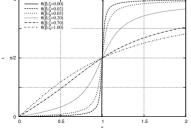
$\theta(\beta,\zeta)$  has a sharper variation around  $\beta=1$  for decreasing values of  $\zeta$ , but it is apparent that, in the case of slightly damped structures, the response is approximately in phase for low frequencies of excitation, and in opposition for high frequencies. It is worth mentioning that for  $\beta=1$  we have that the response is in perfect quadrature with the load: this is very important to detect resonant response in dynamic tests of structures.
