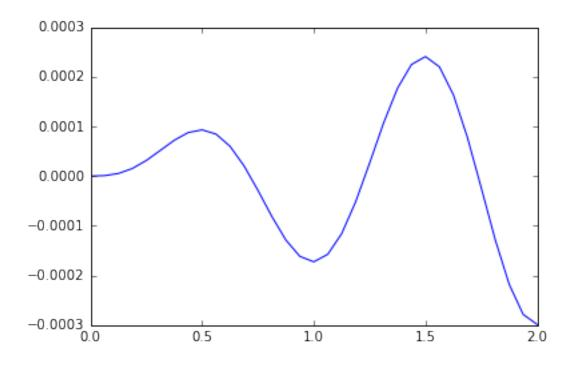
As you can see, the max difference is about 0.3 mm, to be compared with a max response of almost 25 mm, hence an error in the order of 1.2% that in the previous plot led to the apparent disappearance of the NSTEP=16 curve.
