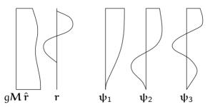
For EQ loading,  $\Gamma_1$  is relatively large for the first mode, as loading components and displacements have the same sign, with respect to other  $\Gamma_i$ 's, where the oscillating nature of the higher eigenvectors will lead to increasing cancellation.
