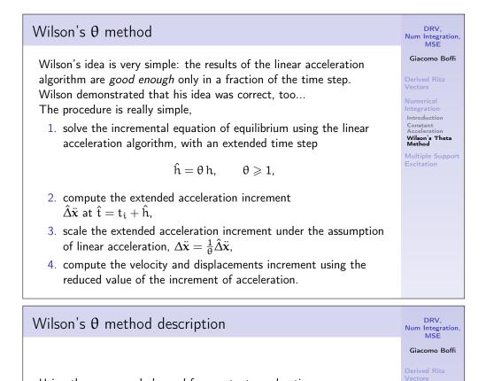
Using the same symbols used for constant acceleration. First of all, for given initial conditions  $x_0$  and  $\dot{x}_0$ , initialise the procedure computing the constants (matrices) used in the following procedure and the initial acceleration,
