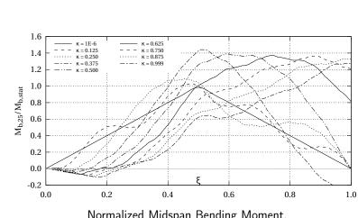
Normalized Midspan Bending Moment. (for different velocities  $v = \kappa v_c$ )
