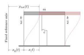
Displacements, deformations and stresses in a structure are induced also by a motion of its support.
