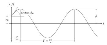
It is worth noting that the coefficients A, B and C have the dimension of a length, the coefficient  $\omega_n$  has the dimension of the reciprocal of time and that the coefficient  $\phi$  is an angle, or in other terms is adimensional.
