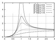
It is possible to measure the support displacement measuring the deflection of the oscillator, within an almost constant scale factor, for excitation frequencies larger than SDOF linear oscillator
