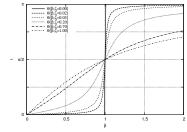
$\theta\left(\beta,\zeta\right)$  has a sharper variation around  $\beta=1$ for decreasing values of  $\zeta$ , but it is apparent that, in the case of slightly damped structures, the response is approximately in phase for low frequencies of excitation, and in opposition for high frequencies. It is worth mentioning that for  $\beta = 1$  we have that the response is in perfect quadrature with the load: this is very important to detect resonant response in dynamic tests of structures.
