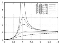
Consider now a harmonic displacement of the support,  $u_g(t) = u_g \sin \omega t$ . The support acceleration (disregarding the sign) is  $a_{\sigma}(t) = \omega^2 u_{\sigma} \sin \omega t$ .
