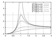
It is possible to measure the support displacement measuring the deflection of the oscillator, within an almost constant scale factor, for excitation frequencies larger than wn.
