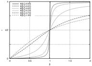
$\theta(\beta,\zeta)$  has a sharper variation around  $\beta=1$  for decreasing values of  $\zeta$ , but it is apparent that, in the case of slightly damped structures, the response is approximately in phase for low frequencies of excitation, and in opposition for high frequencies. It is worth mentioning that for  $\beta=1$  we have that the response is in perfect quadrature with the load: this is very important to detect resonant response in dynamic tests of structures.
