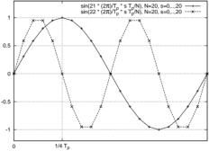
See the plot above: the contributions from the high frequency sines, *when sampled*, are indistinguishable from the contributions from lower frequency components, i.e., are *aliased* to lower frequencies!
