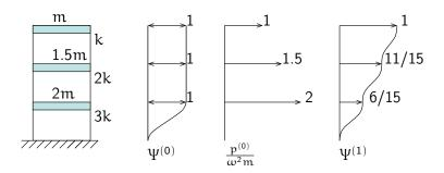
$$\begin{split} T &= \frac{1}{2}\omega^2 \times 4.5 \times m \ Z_0 \\ V &= \frac{1}{2} \times 1 \times 3k \ Z_0 \\ \omega^2 &= \frac{3}{9/2}\frac{k}{m} = \frac{2}{3}\frac{k}{m} \end{split} \qquad \begin{split} \nu^{(1)} &= \frac{15}{4}\frac{m}{k}\omega^2 \Psi^{(1)} \\ \bar{Z}^{(1)} &= \frac{15}{4}\frac{m}{k}\omega^2 \Psi^{(1)} \\$$
