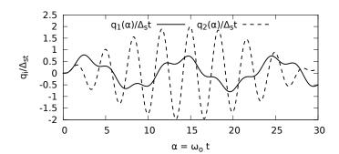
In the graph above, the responses are plotted against an adimensional time coordinate  $\alpha$  with  $\alpha = \omega_0 t$ , while the ordinates are adimensionalised with respect to  $\Delta_{\mathsf{st}} = \frac{p_0}{k}$
