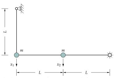
The dynamic system in figure is composed of a single, simply supported uniform beam of negligible mass and two dimensionless bodies, both of mass equal to m; neglecting the axial deformability of the beam the dynamic degrees of freedom are the two vertical displacements of the bodies,  $x_1$  and  $x_2$ .
