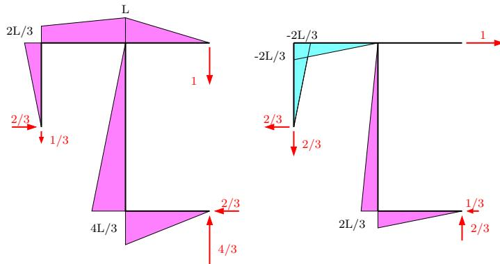
the stiffness is computed by inversion and the mass matrix is the unit matrix multiplied by  $m$ ,  $\mathbf{M} = m \mathbf{I}$ .
