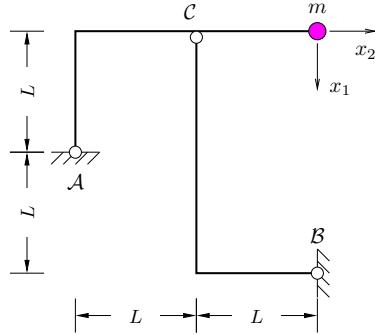
The dynamical system in figure is composed of two massless, uniform beams supporting a dimensionless body of mass  $m$ .
