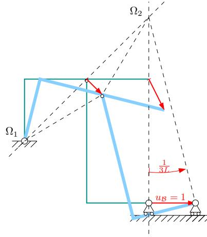
The angle of rotation of the lower beam is  $\theta_2 = 1/3L$ , anti-clockwise and the angle of rotation of the upper beam (that rotates about the hinge in  $\mathcal{A}$ ) is equal but clockwise, due to the continuity of displacements in the internal hinge  $\mathcal{C}$ .
