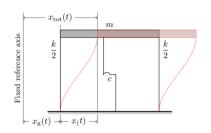
Considering a support motion  $x_{\rm g}(t)$ , defined with respect to a inertial frame of reference, the total displacement is
