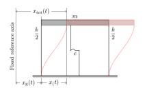
Considering a support motion  $x_{\rm g}(t)$ , defined with respect to a inertial frame of reference, the total displacement is
