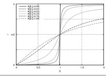
$\theta(\beta,\zeta)$  has a sharper variation around  $\beta=1$  for decreasing values of  $\zeta,$  but it is apparent that, in the case of slightly damped structures, the response is approximately in phase for low frequencies of excitation, and in opposition for high frequencies. It is worth mentioning that for  $\beta=1$  we have that the response is in perfect quadrature with the load: this is very important to detect resonant response in dynamic tests of structures.
