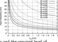
Knowing the frequency of excitation and the required level of vibration isolation efficiency (IE), one can determine the minimum static deflection (proportional to the spring flexibility) required to achieve the required IE. It is apparent that any isolation system must be very flexible to be effective.
