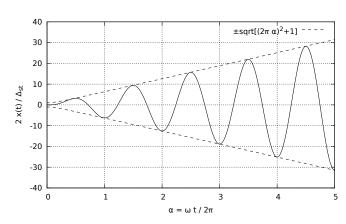
$\frac{2}{\Delta_{\rm st}} x(t) = \sin \omega t - \omega t \cos \omega t = \sin 2\pi \alpha - 2\pi \alpha \, \cos 2\pi \alpha.$
