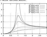
It is possible to measure the support displacement measuring the deflection of the oscillator, within an almost constant scale factor, for excitation frequencies larger than  $\omega_{\rm n}$ .
