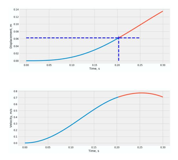
In the next phase, still it is  $\dot{x} > 0$  so that the spring is still yielding, but now p(t) = 0, so we must compute two new state functions, starting as usual from the initial conditions (note that the yielding force is still applied)
