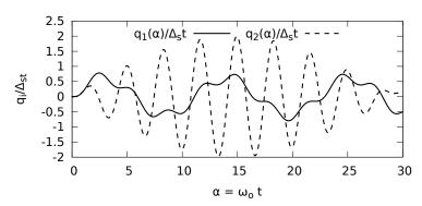
In the graph above, the responses are plotted against an adimensional time coordinate  $\alpha$  with  $\alpha = \omega_0 t$ , while the ordinates are adimensionalised with respect to  $\Delta_{\mathsf{st}} = \frac{p_0}{k}$
