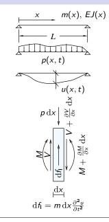
At the left, a straight beam with characteristic depending on position x: m = m(x) and EJ = EJ(x); with the signs conventions for displacements, accelerations, forces and bending moments reported left, the equation of vertical equilibrium for an infinitesimal slice of beam is
