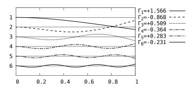
Above, the modal mass decomposition  $r_n = \Gamma_n m \phi_n$ , for the first six modes of a uniform cantilever, in abscissa x/L.
