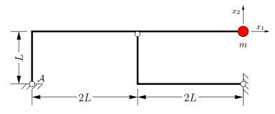
The dynamic system in figure is composed of two uniform beams of negligible mass, their flexural stiffness being EJ = const, supporting a lumped mass of negligible rotatory inertia (the flexibility matrix is  $\mathbf{F} = \frac{L^3}{6EJ} \begin{bmatrix} 3 & 2\\ 2 & 96 \end{bmatrix}$ ).
