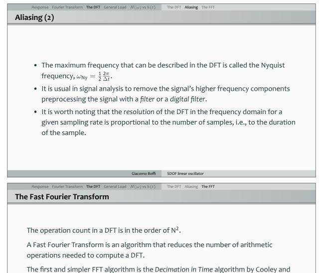
The first and simpler FFT algorithm is the *Decimation in Time* algorithm by Cooley and Tukey (1965).
